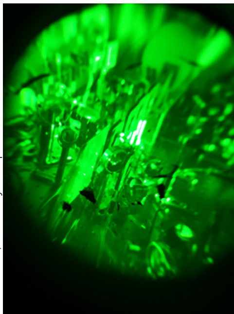
Part of the many optics of the multipass amplifier passing the laser at 800 mJ (photo taken through an infrared telescope).
